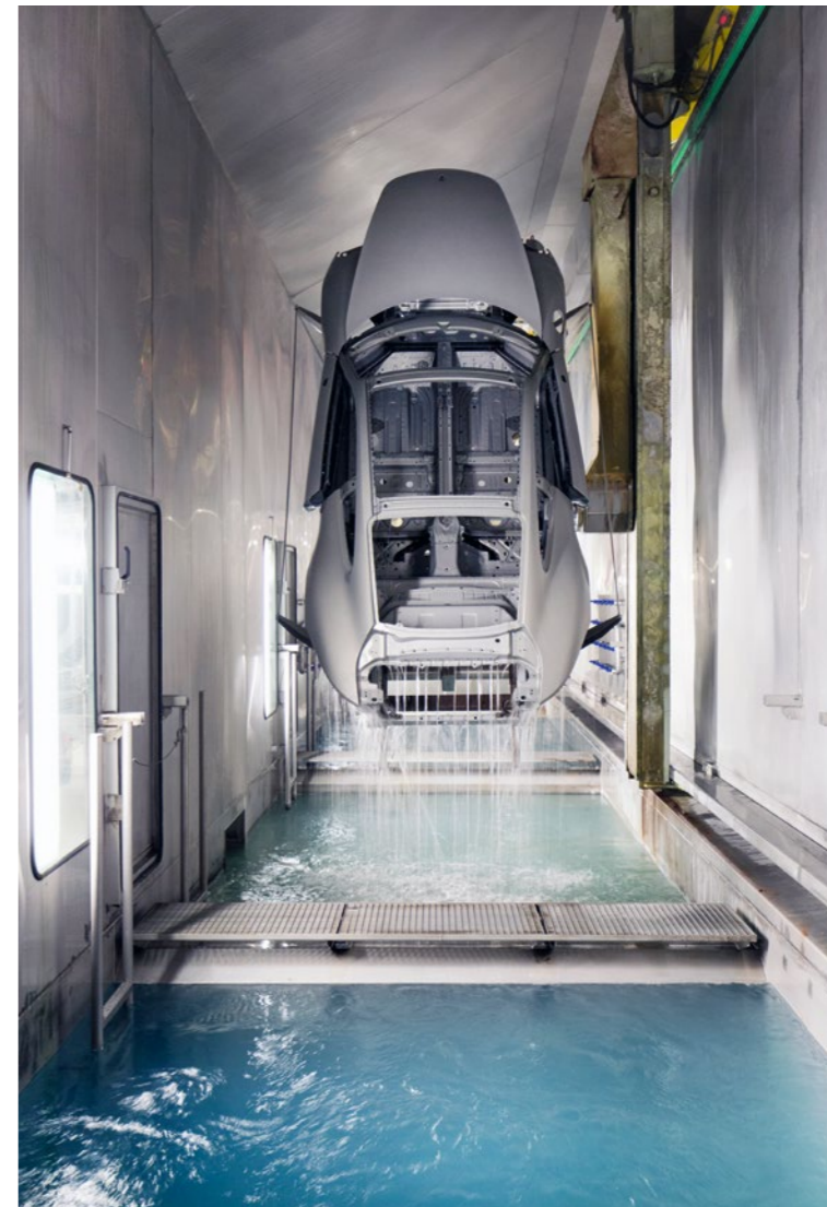
PRE-TREATMENT PROCESS IN PAINT SHOP
