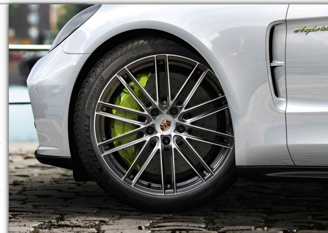
Porsche Ceramic Composite Brake (PCCB)
