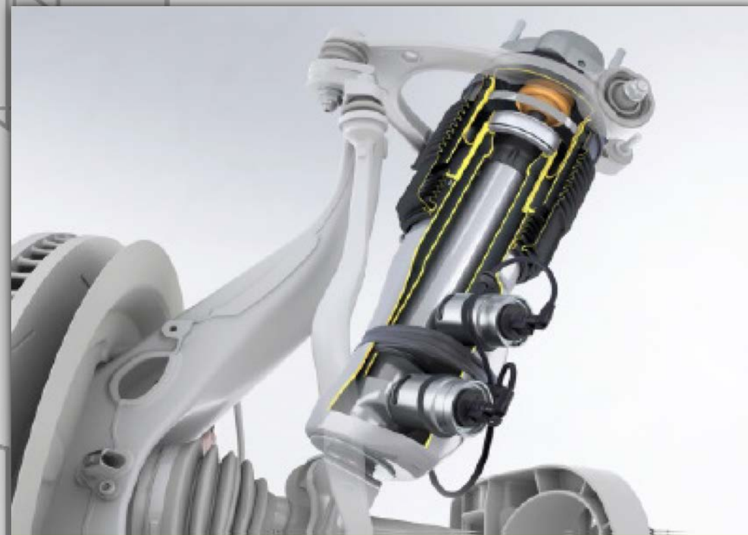
3-chamber air suspension
